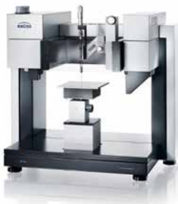
2. Figure. Krüss DSA 100 drop shape analyser [ 3 ]
