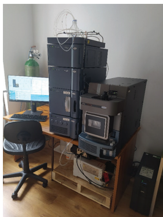
Figure 1 Waters Acquity UPLC-TQS micro tandem quadrupole mass spectrometer
